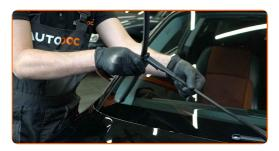
Remove the blade from the wiper arm.
