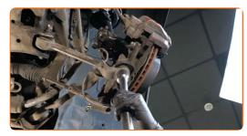
Tighten the rear fastener of the control arm. Use a combination spanner #18. Use a drive socket #18. Use a torque wrench. Tighten it to 68 Nm torque.+90°
