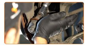
Install the brake caliper together with its bracket.
