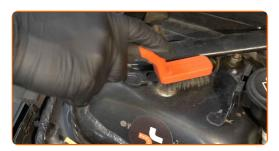
Loosen the upper fastener of the shock strut mount. Use a combination spanner #13.
