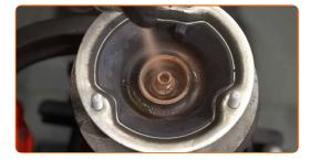
Install the shock strut mount cap.
