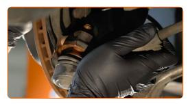
Screw on the fastening nut that connects the tie rod end to the steering knuckle. Use a drive socket #21. Use a ratchet wrench.
