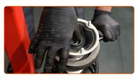
Tighten the shock strut piston rod nut. Use a drive socket #21. Use HEX No.H6. Use a torque wrench. Tighten it to 64 Nm torque.
