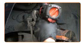
Treat all joints of the arm. Treat the shock strut fasteners. Use copper grease.
