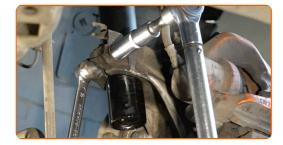
Remove the support from under the arm.
