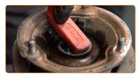
Remove the strut piston rod nut. Use a drive socket #21. Use HEX No.H6. Use a ratchet wrench.
