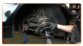
36 Set the shock absorber strut on the spring compressor tool.
