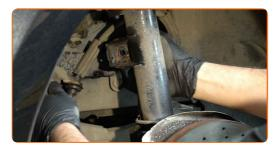
Disconnect the ABS sensor wiring.
