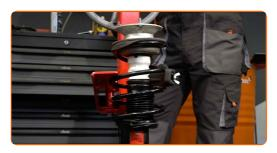
Remove the assembled shock strut.
