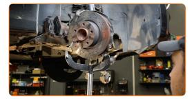
Release the lower fastener connecting the shock strut to the steering knuckle. Use a special drive socket to remove the shock absorber. Use a ratchet wrench.
