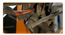
Unscrew the end fastening nut to the steering knuckle. Use a drive socket #21. Use a ratchet wrench.
