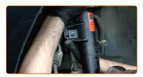
Tighten the fastener connecting the stabilizer link to the shock strut. Use a combination spanner #18. Use a drive socket #15. Use a torque wrench. Tighten it to 58 Nm torque.
