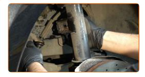
Disconnect the ABS sensor wiring.
