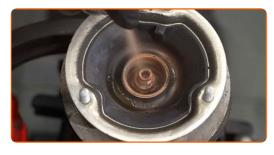
Install the shock strut mount cap.
