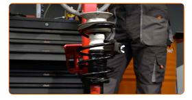
Remove the assembled shock strut.
