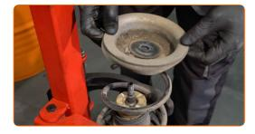
Release the coil spring.
