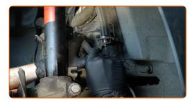
Connect the ABS sensor wiring.
