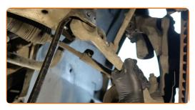
Remove the fastening bolt.
