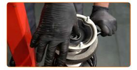
Tighten the shock strut piston rod nut. Use a drive socket #21. Use HEX No.H6. Use a torque wrench. Tighten it to 64 Nm torque.
