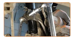
Remove the support from under the arm.
