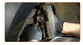
Disconnect the ABS sensor wiring.
