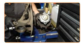
Clean the wheel hub mounting seat. Use a wire brush. Use WD-40 spray.
