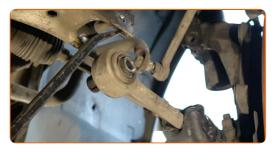
Remove the fastening bolt.
