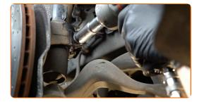
Unscrew the front arm fastener. Use a combination spanner #18. Use a drive socket #18. Use a ratchet wrench.
