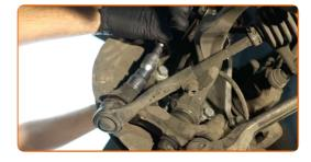
64 Attach the ABS sensor connector.
