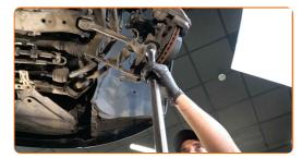
Tighten the rear fastener of the control arm. Use a combination spanner #18. Use a drive socket #18. Use a torque wrench. Tighten it to 68 Nm torque.+90°
