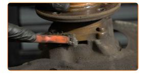
Unscrew the wheel hub axle nut. Use a drive socket #18. Use a ratchet wrench.
