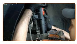
Tighten the fastener connecting the stabilizer link to the shock strut. Use a combination spanner #18. Use a drive socket #15. Use a torque wrench. Tighten it to 58 Nm torque.
