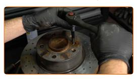
Remove the brake disc.
