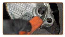
Treat the wheel hub mounting seat. Use copper grease.
