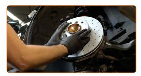
Tighten the brake disc fastening. Use HEX No.H6. Use a torque wrench. Tighten it to 9 Nm torque.
