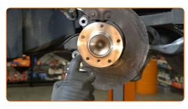
23 Install the brake disc.
