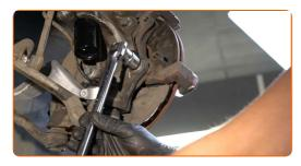
18 Remove the caliper bracket.
