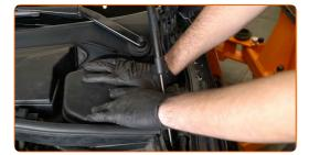
Remove the fender protection cover. Close the hood.
