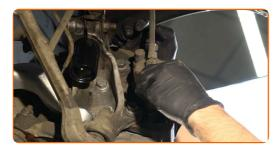
Install the brake caliper retaining spring.
