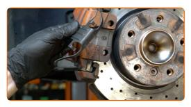
Remove the brake caliper.
