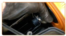
Reinstall the air filter cover. Fasten it.
