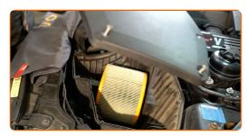
Detach the air duct housing from the air filter housing. Use a flat screwdriver.
