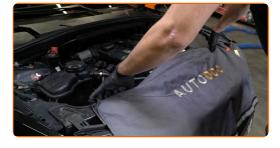
Undo the fastening screws of the air filter cover. Use Torx T25. Use a ratchet wrench.
