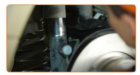
Remove the support from under the stub axle.
