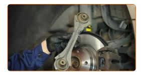
Clean the mounting seats and the thread of the suspension arm. Use a wire brush. Use WD-40 spray.
