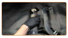
Remove the shock absorber mount, boot and bump stop.
