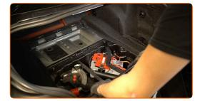
Screw in the fastener of the central protective plastic panel. Use a Phillips screwdriver. Use Torx T40. Use a ratchet wrench.
