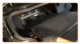
Unscrew the fastener of the central protective plastic panel. Use a Phillips screwdriver. Use a clip removal tool. Use Torx T40. Use a ratchet wrench.
