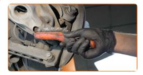
Unscrew the lower fastener of the shock absorber. Use a drive socket #14. Use a ratchet wrench.
