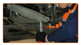
Tighten the lower fastener of the shock absorber. Use a drive socket #E12. Use a torque wrench. Tighten it to 47 Nm torque.
