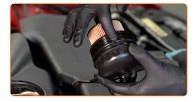
Screw the new filter into its place.
