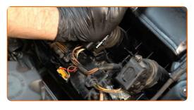
Install the engine cover and secure it.
