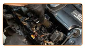
Plug in the ignition coil connector.
