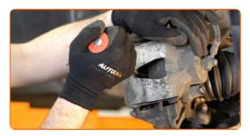
10 Remove the brake caliper.
