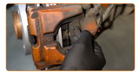
Disconnect the brake pads wear sensor.
