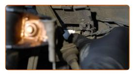
13 Install the wear sensor on the brake pads.
