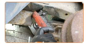
Treat the shock absorber mounting seats. Use copper grease.
