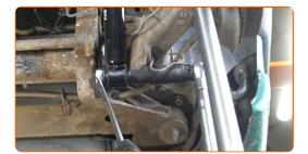
Tighten the top shock absorber fastening. Use a drive socket #24. Use a torque wrench. Tighten it to 110 Nm torque.
