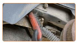
Unscrew the upper fastener of the shock absorber. Use a drive socket #24. Use a ratchet wrench.
