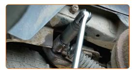
Unscrew the lower fastener of the shock absorber. Use a combination spanner #24. Use a drive socket #24. Use a ratchet wrench.
