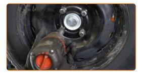
Lower the car and working in a cross order, tighten the wheel bolts. Use wheel impact socket #19. Use a torque wrench. Tighten it to 90 Nm torque.
