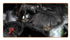
Remove the fuel filter housing cover.
