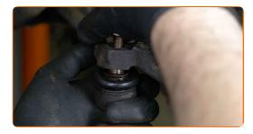
Tighten the fastening nut connecting the tie rod end to the steering knuckle. Use a drive socket #17. Use a torque wrench. Tighten it to 40 Nm torque.
