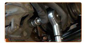
79 Install the brake hose bracket.
