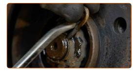
9 Remove the circlip.
