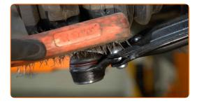
Unscrew the lower fastener connecting the shock strut to the steering knuckle. Use a combination spanner #16. Use a drive socket #16. Use a ratchet wrench.
