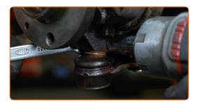
Screw in the fastener that connects the shock strut to the steering knuckle. Use a combination spanner #16. Use a drive socket #16. Use a ratchet wrench.
