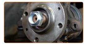
Screw the nut of the drive shaft. Use a drive socket #36. Use a ratchet wrench.
