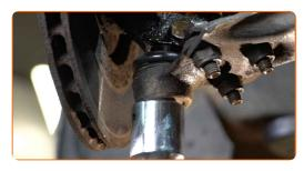
Unscrew the fastener connecting the ball joint to the suspension control arm. Use a combination spanner #16. Use a drive socket #16. Use a ratchet wrench.
