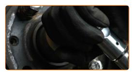
Restake the fastener of the driveshaft. Use a flat metal-working chisel. Use a hammer. 45
