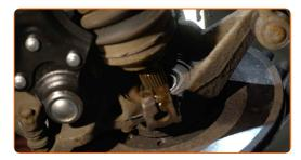
Treat the ball joint fastener. Use copper grease.
