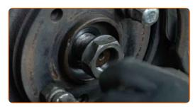
Loosen the CV axle in the wheel hub. Use a pin punch. Use a hammer.
