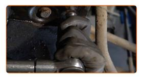
Tighten the rear fastener of the control arm. Use a combination spanner #16. Use a drive socket #16. Use a torque wrench. Tighten it to 90 Nm torque.
