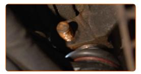
Tighten the fastener connecting the ball joint to the steering knuckle. Use a combination spanner #16. Use a drive socket #16. Use a torque wrench. Tighten it to 40 Nm torque.
