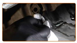
Screw in the new drainage plug and tighten it. Use a drive socket #24. Use a torque wrench. Tighten it to 28 Nm torque.
