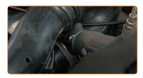
17 Remove the fender protection cover.
