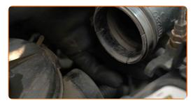
6 Release the air filter cover clips.
