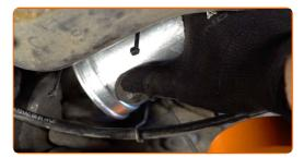
Attach the fuel filter fasteners. Use nippers.
