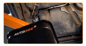
Squeeze the clips and detach the fuel supply lines from the fuel filter housing. Use a flat screwdriver.
