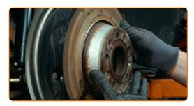
Remove the hub bearing protection cap. Use a hammer. Use a crowbar.
