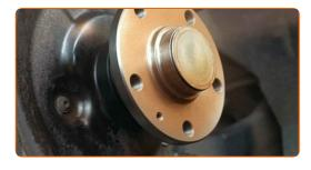
30 Install the brake disc.
