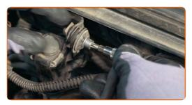
6 Unscrew the brake fluid reservoir cap.
