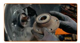
Clean the hub bearing mounting seat. Use a wire brush. Use all-purpose cleaning spray.
