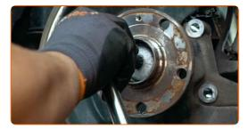
Remove the fastening bolt.
