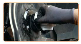
Install the new wheel hub with a bearing. Use a bush and bearing driver set. Use a hammer.
