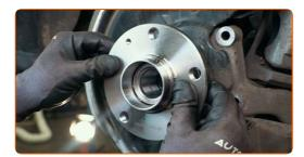
Treat the fasteners of the wheel hub bearing. Use a sealant.
