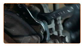
Remove the brake caliper.
