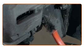
Unscrew the brake caliper fastening. Use a combination spanner #13. Use a combination spanner #15. Use a drive socket #13. Use a ratchet wrench.
