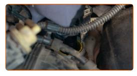
Install the engine solenoid valve bracket. Use Torx T27. Use a ratchet wrench.
