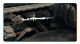
Unscrew the brake fluid reservoir cap.
