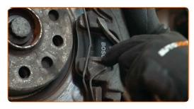
14 Remove the brake caliper.
