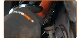
Unscrew the fastener connecting the stabilizer link to the shock strut. Use a drive socket #18. Use a ratchet wrench.
