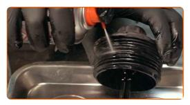
Install new O-rings and a new oil filter to their mounting seats on the filter cover.
