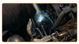
Screw in the bracket for the engine pipes. Use Torx T30. Use a ratchet wrench.
