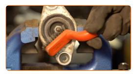
Remove the shock absorber piston rod fastening. Use a combination spanner #17. Use an adjustable wrench.
