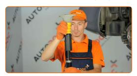
Tighten the shock absorber rod nut. Use a combination spanner #16. Use an adjustable wrench. Use a torque wrench. Tighten it to 25 Nm torque.
