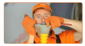
Remove the shock absorber mount, boot and bump stop. Use a rubber mallet.
