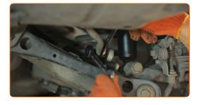
Remove the fastening bolt.
