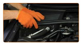
Remove the fender protection cover.
