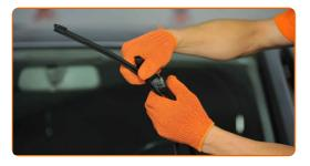
Remove the blade from the wiper arm.
