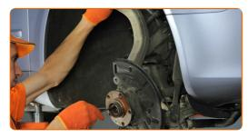
Remove the steering knuckle together with the hub. Use a flat screwdriver.
