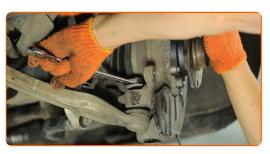
Tighten the ball joint fastener. Use a combination spanner #18. Use a torque wrench. Tighten it to 110 Nm torque.
