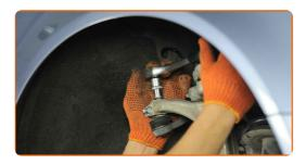
Tighten the fastening nut connecting the tie rod end to the steering knuckle. Use a drive socket #16. Use a torque wrench. Tighten it to 45 nm torque.
