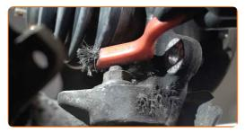
Unscrew the ball joint fastening to the steering knuckle. Use a combination spanner #18.
