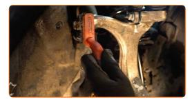
Unscrew the end fastening nut to the steering knuckle. Use a drive socket #13.
