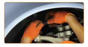
Connect the ABS sensor wiring. Use a flat screwdriver.
