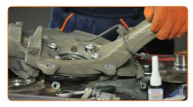
Tighten the fastener of the wheel hub bearing. Use XZN #12. Use a torque wrench. Tighten it to 80 Nm torque.+90°
