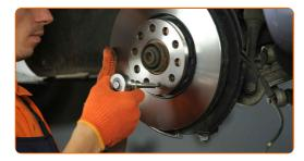
16 Remove the brake disc.
