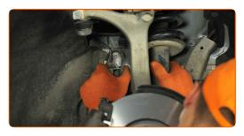
Attach the ABS sensor connector.
