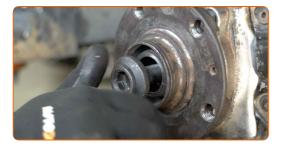
Tighten the hub. Use HEX No.H17. Use a torque wrench. Tighten it to 115 Nm torque.+180°
