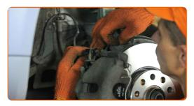
67 Connect the ABS sensor wiring.
