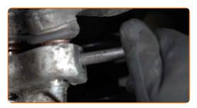
Detach the upper control arm from the steering knuckle. Use a flat metal-working chisel. Use a hammer.
