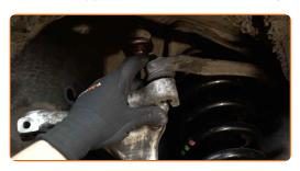
Install the fastening bolt. Use a hammer. Use a pin punch.
