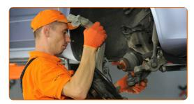
Press the wheel hub out from the tapered roller bearing. Use a bush and bearing driver set. Use a hammer.
