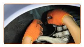
9 Disconnect the ABS sensor wiring.
