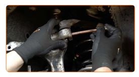
Tighten the upper arm fastenings. Use a combination spanner #16. Use a drive socket #16. Use a torque wrench. Tighten it to 40 Nm torque.
