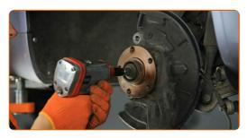
19 Remove the fastening bolt.
