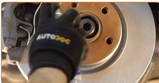
**45** Clean the brake disk surface. Use a brake cleaner.
