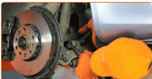
**15** Unscrew the fastener connecting the stabilizer link to the stabilizer bar. Use a combination spanner #16.
