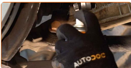
**44** Treat the surface where the brake disc contacts the wheel rim. Use copper grease.
