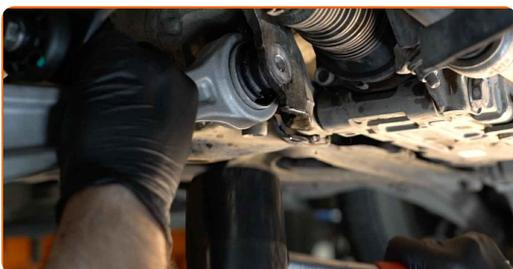
**30** Install the fastening bolt. Use a hammer. Use a pin punch.
