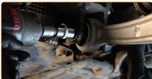
**32** Attach the bottom part of the shock strut.
