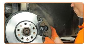
Use HEX No.H7. Use a torque wrench. Tighten it to 30 Nm torque.
