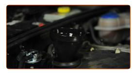
Pour oil into the engine through the filler. Required amount of oil: 3,8 L.
