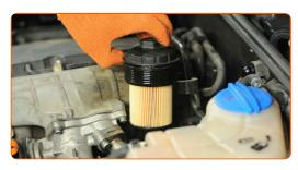
Use a drive socket #32. Use a torque wrench. Tighten it to 25 Nm torque.
