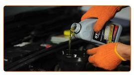
Replacement: engine oil and filter – Audi A4 B7 Avant. Tip from AUTODOC experts:
