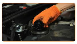
Tighten the oil filler cap.
