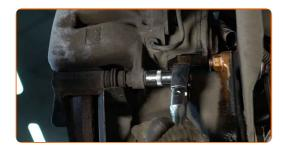
10 Remove the brake caliper.
