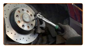
Tighten the fastener of the wheel hub bearing. Use XZN #16. Use a torque wrench. Tighten it to 200 Nm torque.+180°
