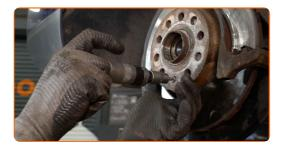
Remove the brake disc.
