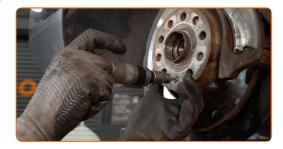
16 Remove the brake disc.
