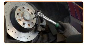
Tighten the fastener of the wheel hub bearing. Use XZN #16. Use a torque wrench. Tighten it to 200 Nm torque.+180°
