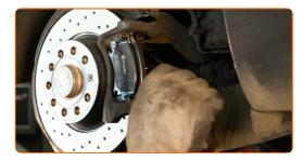
Treat the brake caliper piston. Use a wire brush. Use a brake cleaner.
