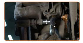
11 Remove the brake caliper.
