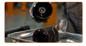
Detach the oil filter from the filter cover.
