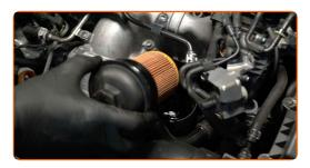
Install a new oil filter housing cover and tighten it. Use a drive socket #32. Use a torque wrench. Tighten it to 25 Nm torque.
