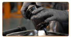
17 Remove the oil filter cover O-ring. Use a flat screwdriver.
