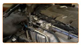
Move the vacuum system components aside.
