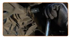
Unscrew the rear fastener connecting the control arm to the car body. Use a drive socket #18. Use a tap wrench.
