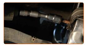
Install the rear fastener of the control arm (2 pieces).
