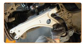
Screw the front arm fastener. Use a drive socket #18. Use a ratchet wrench.
