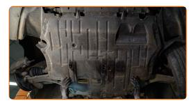
Tighten the fasteners of the oil pan lower cover. Use a drive socket #13. Use Torx T25. Use a ratchet wrench.
