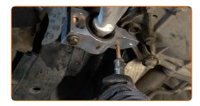
Tighten the fasteners of the ball joint. Use a drive socket #16. Use a torque wrench. Tighten it to 60 nm torque.
