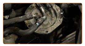
Tighten the fasteners of the fuel filter housing cover. Use Torx T20. Use a ratchet wrench. Use a torque wrench. Tighten it to 9 nm torque.
