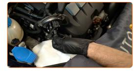
Remove the microfibre cloth from the fuel filter housing.
