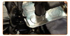
8 Cover the fuel filter housing with a microfibre cloth to prevent dirt and foreign objects from getting into the system.
