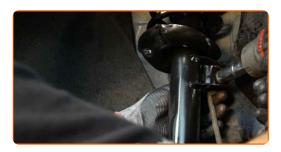
Unscrew the fastener connecting the stabilizer link to the stabilizer bar. Use a combination spanner #18. Use HEX No.H5. Use a ratchet wrench.
