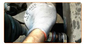
Tighten the fastener connecting the stabilizer link to the shock strut. Use a combination spanner #18. Use a drive socket #18. Use a torque wrench. Tighten it to 65 Nm torque.
