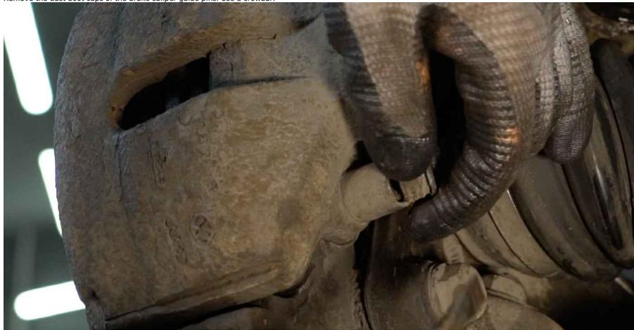
9 Unscrew the brake caliper fastening. Use HEX No.H7. Use a ratchet wrench.
