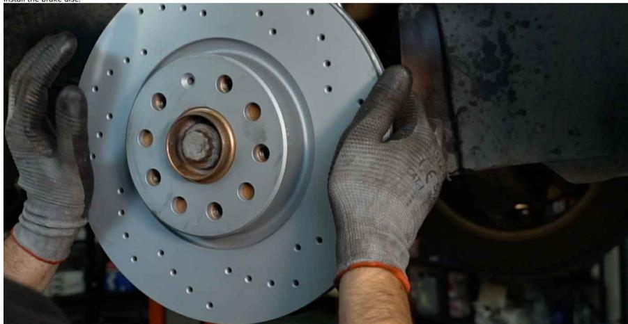
21 Tighten the brake disc fastening. Use Torx T30. Use a torque wrench. Tighten it to 4 Nm torque.
