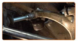
25 Tighten the fastening nut connecting the tie rod end to the steering knuckle. Use a drive socket #13. Use a torque wrench. Tighten it to 7 nm torque.
