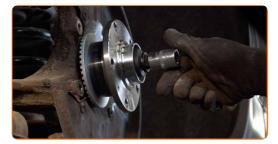
Tighten the fastener of the wheel hub bearing. Use HEX No.H19. Use a torque wrench. Tighten it to 200 Nm torque.+180°
