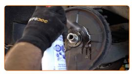
21 Install the new wheel hub with a bearing.
