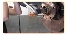
18 Remove the fastening bolt.
