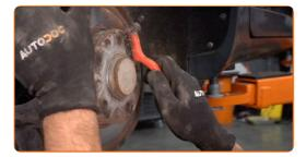
Remove the retaining ring. Use a crowbar.
