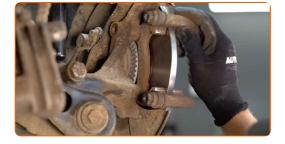
Tighten the brake caliper bracket. Use HEX No.H8. Use a torque wrench. Tighten it to 75 Nm torque.
