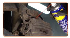
9 Unscrew the brake caliper fastening. Use a combination spanner #13. Use a combination spanner #15.
