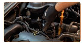
Install a new oil filter housing cover and tighten it. Use the 76-14F socket. Use a torque wrench. Tighten it to 25 Nm torque.
