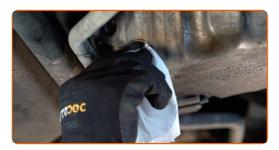
Screw in the new drainage plug and tighten it. Use a drive socket #19. Use a torque wrench. Tighten it to 30 Nm torque.
