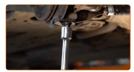
Tighten the fastener connecting the stabilizer link to the stabilizer bar. Use a combination spanner #16. Use a drive socket #16. Use a torque wrench. Tighten it to 40 Nm torque.+90°
