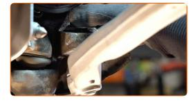
Screw the fasteners of the ball joint. Use a combination spanner #18. Do not tighten it.
