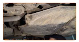
Tighten fixing bolts of the protective cover. Use a flat screwdriver.
