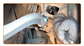
Treat all joints of the arm. Use a multipurpose grease. Use a flat screwdriver.
