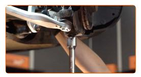
Tighten the rear fastener connecting the control arm to the subframe. Use a combination spanner #18. Use a drive socket #18. Use a torque wrench. Tighten it to 70 Nm torque.+180°
