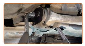
Unscrew and remove the wheel arch cover fasteners. Use a Phillips screwdriver. Use a drive socket #10. Use a ratchet wrench.
