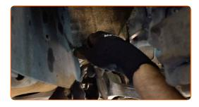
Remove the fastening bolt. Use a crowbar.
