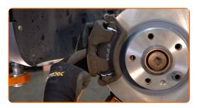
Connect the brake pads wear sensor.
