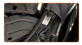
Detach the air intake hose clamp. Use a drive socket #7.
