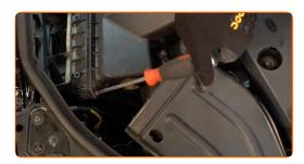
Remove the air intake hose Use Torx T20.
