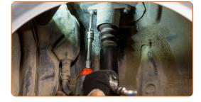
Attach the lower part of the shock absorber.
